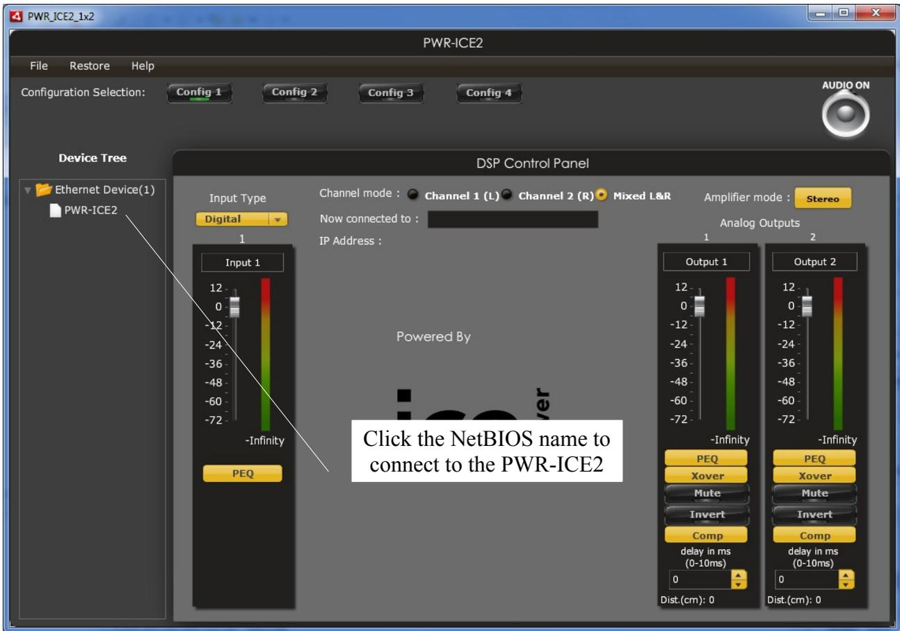
6. The PWR-ICE2 device will be connected with its NetBIOS name and IP address displayed at the middle of the plugin.
