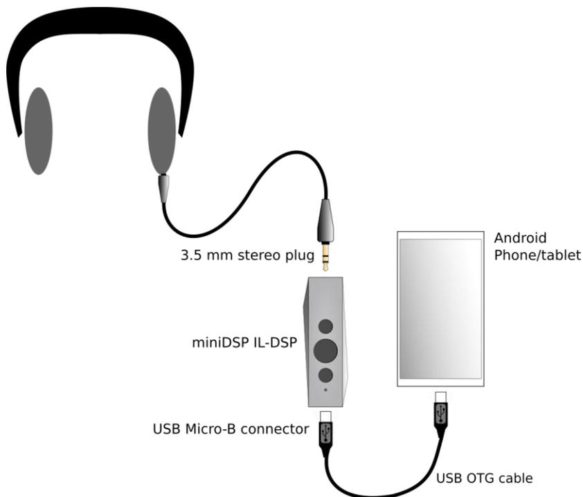
1. Use one of the supplied OTG cables to connect your phone or tablet, depending on whether your Android device has a USB-C or Micro USB B socket.
