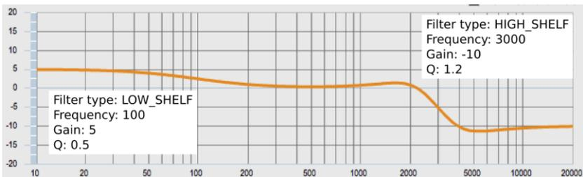
On the right side, we have used a high shelf filter with negative gain to cut high frequencies by about 10 dB. The Q shown is higher than you usually use for this type of filter.
