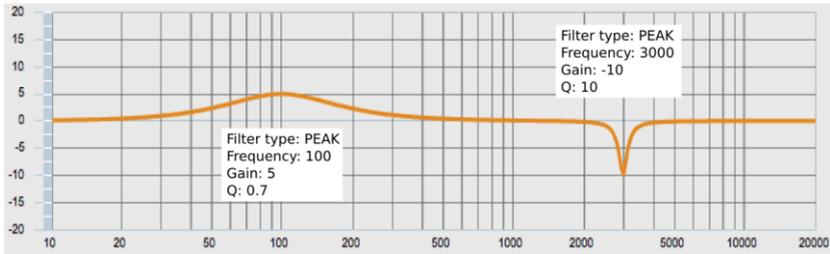
If the gain is negative, the filter cuts a frequency range. On the right side above we have used negative gain, with a narrow frequency range set by using a high value of Q.
