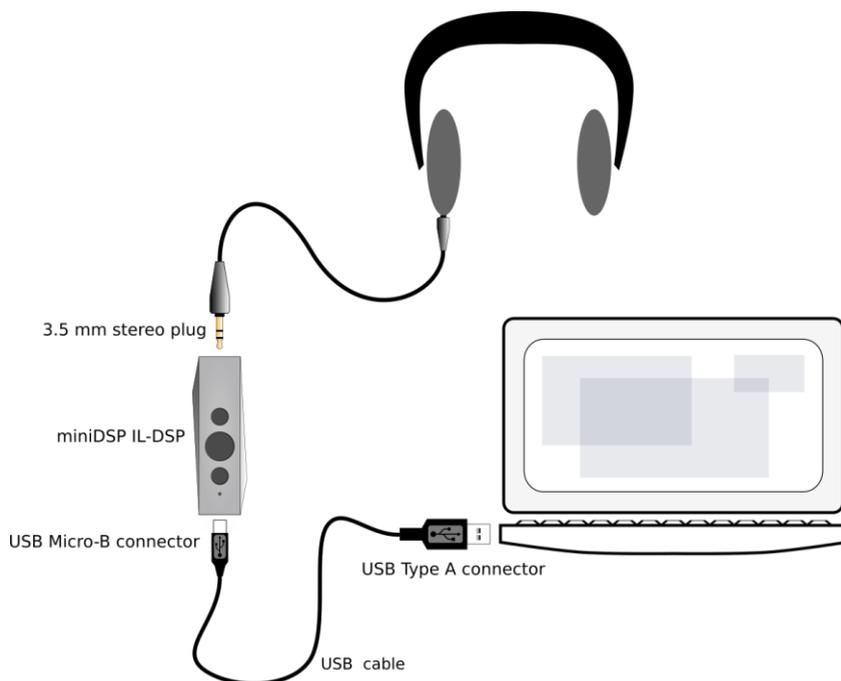
1. Connect the USB cable supplied with the IL-DSP to a USB port on your computer.
